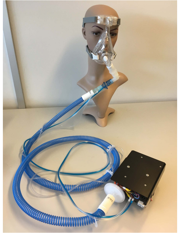
Fig. 2. Photograph of a respiratory system with a hose that connects to a patient.
