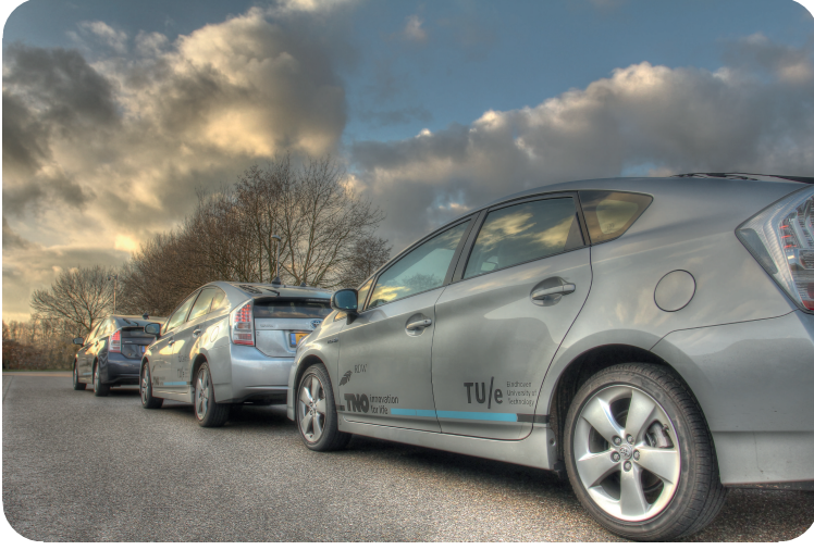
Figure 3.13: Experimental vehicle platoon, consisting of three CACC-equipped passenger vehicles.
