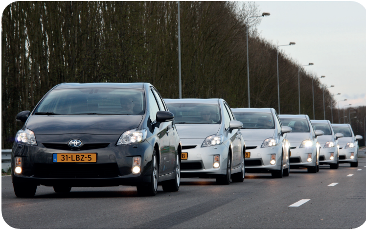
Figure 2.5: Test fleet, consisting of CACC-equipped passenger vehicles.
